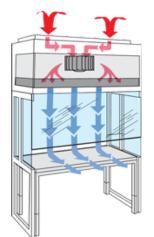
Room air (in red) enters the system from above the HEPA filter; 99.99% particle-free air is forced downward toward the work surface.
