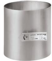
**3858800—Backdraft Damper.** Mounts in vertical duct run to prevent reverse pressurization of the exhaust system. 3.0" (8 cm) high with 10" (25.4 cm) dia. OD inlet and outlet. Shipping weight 5.0 lbs. (2.0 kg)
