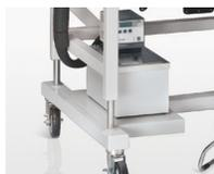
**3784000—Caster Kit.** Includes four 5" (13 cm) dia., non-marking polyurethane casters with toe locks and bearings. Load rating for each caster is 250 lbs. Casters replace the fixed feet and add 11" (28 cm) to the overall depth of base stand. **Installation is required.\*\*** Not for use with stands that support Type B2 BSC. Shipping weight 10 lbs. (5 kg)
