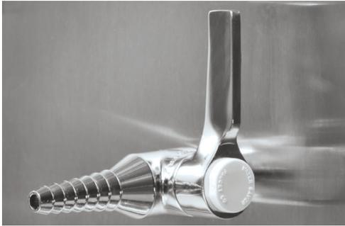
**Service Fixture.** Ball-type valve supplies water, vacuum, air or noble gases to cabinet interior. Serrated tip with quarter turn handle is mounted 8.5" (20 cm) above the work surface to maximize usable surface area. Max 40 psi. Accessory Package includes one right-hand service fixture (3', 4', and 5' models) or one service fixture on each side (6' models).
