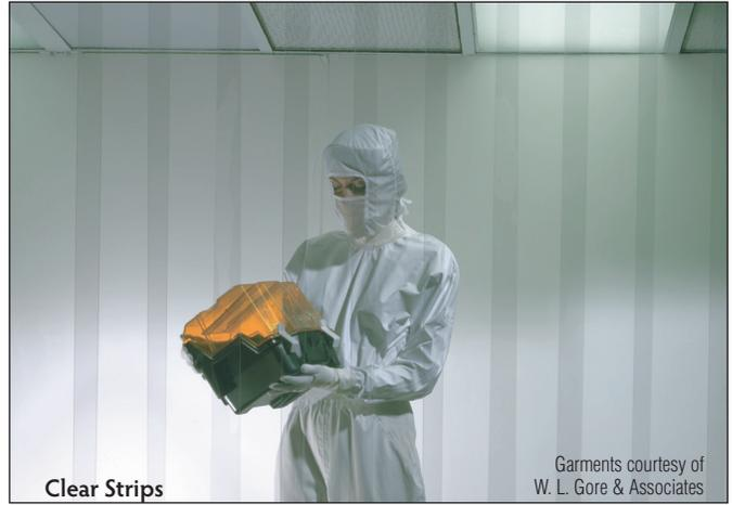
Select the panel material to meet your application requirements. Static-Dissipative PVC includes permanent built-in static inhibitors that, unlike topical treatments, will not wear off. Tests performed per ASTM D257 show surface resistivity of  $1.8 \times 10^{10}$  ohms/sq.
