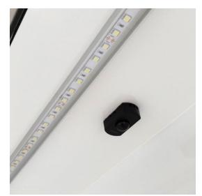
Figure 3. Motion sensor next to the LED light strip
