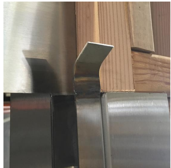
Figure 3: The door tracks on the “dirty side” can be identified by the curved door guides
