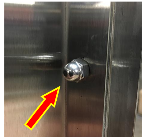
Figure 1: Break down the door frame by removing the cap nuts shown here
