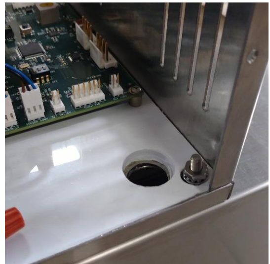
Figure 10: One pass-through hole is located on the opposite side, near the circuit board
