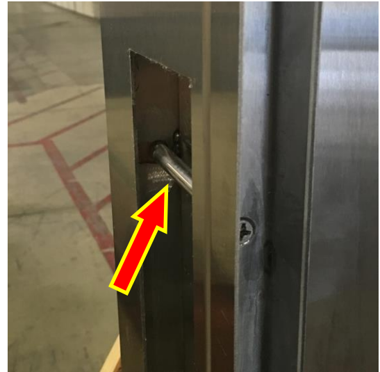
Figure 8: The touch panel side of the frame has internal guides for the 6" screws
